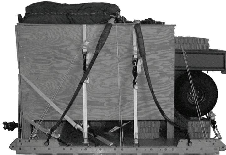
One Military Utility Vehicle (M-Gator) Rigged on an 8-Foot Platform
